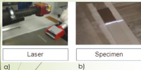
Fig. 14. A laser can be used to prepare the surface before gluing. a) Laser head with hood for removing ablation products b) A sample
