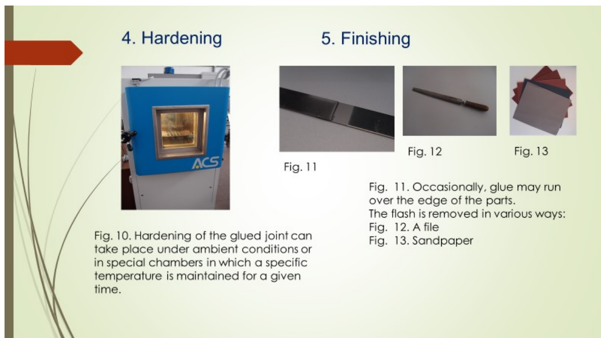
Figure 4.11. Hardening and finishing
