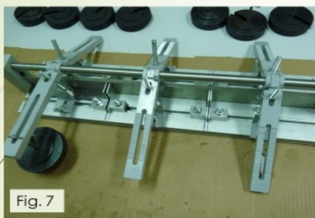
Fig. 7. A special handle for positioning the glued elements Fig. 8. Prepared elements for gluing Fig. 9. Connection made
