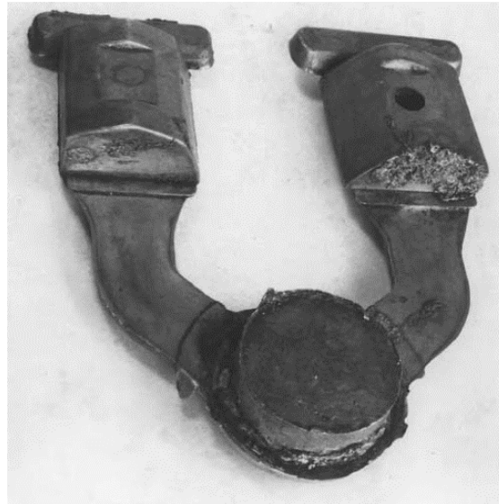
Figure 4.3. Pair of aluminium alloy die castings on common sprue, as removed. Notice the broken skin in the end face at the right-hand side where liquid metal has burst out after dies opened. [4.1]
